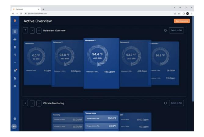
On a (home screen) dashboard, cards allow users to view equipment point values and change setpoints and other control functions. Cards are the primary means to visualize network data and control equipment from a web browser.
