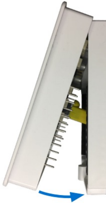
Illustration 7—Reinstalling the Cover on the Backplate
