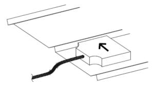
**NOTE:** If the unit has more than one outside air damper, mount the inclinometer on a horizontal-axis return air damper blade. (However, if the unit also has more than one return air damper, an AFMS cannot be installed.)
