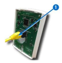
Plug an Ethernet patch cable 1 connected to an STE-9000 Series NetSensor into the (yellow) ROOM SENSOR port 2 of the controller.
