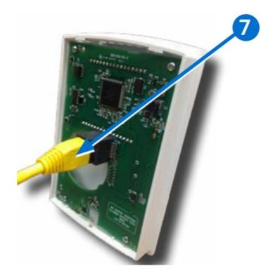
1. Plug an Ethernet patch cable 7 connected to an STE-9000 Series or STE-6010/6014/6017sensor into the (yellow) ROOM SENSOR port 8 of the controller.
