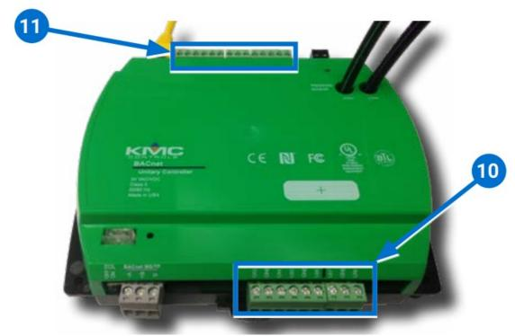
3. Wire additional equipment (such as fans, heaters, dampers, and valves) to the green (output) terminal block 11 . See Sample (BAC-9311) Wiring on page 7.
