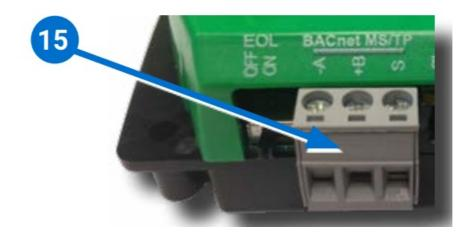
**NOTE:** Use 18 gauge AWG shielded twisted pair cable with the maximum capacitance of 51 picofarads per foot (0.3 meters) for all network wiring (Belden cable #82760 or equivalent).
