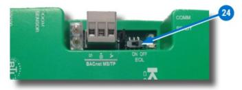
3. If the controller is at either end of a BACnet MS/TP network (only one wire under each terminal), turn the EOL switch 24 to ON.
