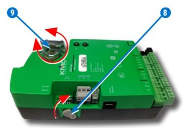
**NOTE:** Continue to rotate the drive hub and V-clamp until they reach a stop.
