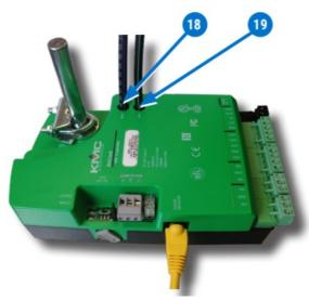
3. Connect the low-pressure tube from the pressure flow sensor to the LOW 19 port on the controller.
