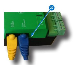
NOTE: The Ethernet patch cable should be T568B Category 5 (or better) and a maximum of 328 feet (100 meters) between devices.
