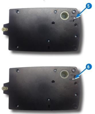
**NOTE:** Overtightening the screw can cause compression in the case which may interfere with the controller's operation.
