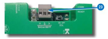
NOTE: Use 18 gauge AWG shielded twisted pair cable with the maximum capacitance of 51 picofarads per foot (0.3 meters) for all network wiring (Belden cable #82760 or equivalent).
