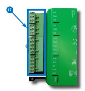
**NOTE:** Wire sizes 12–24 AWG can be clamped in each terminal.
