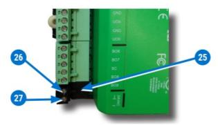
• B. Connect the AC phase side of the transformer to the controller's phase terminal  $\sim 27$ .
