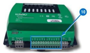
4. Connect equipment to the green (output) terminals 10 . See Sample (BAC-5900A) Wiring on page 8 and BAC-5900A series videos on the KMC Conquest Controller Wiring playlist
