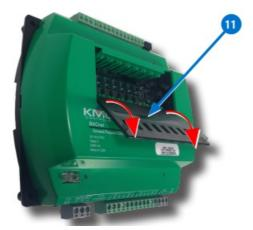
3. Remove the jumper 12 from the slot in which the override board will be installed.
