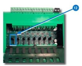
NOTE: Each of the eight override slots ships from KMC with a jumper installed on the two pins closest to the output terminal blocks.\ Only remove a jumper if an override board will be installed
