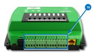
**NOTE:** HPO-6701 triac and HPO-6703/6705 relay board circuits use the Switched Common SC terminal—not the Ground Common GND terminal.
