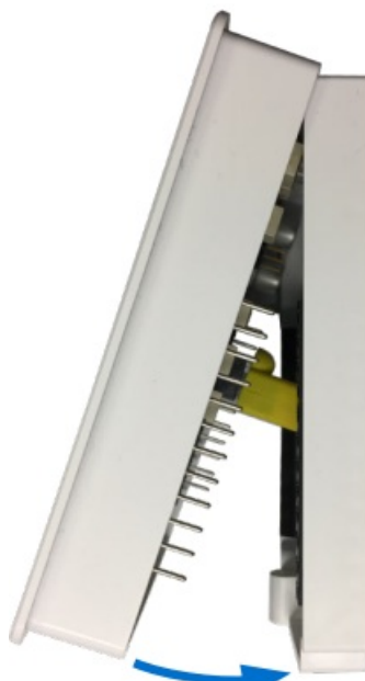
Illustration 7—Reinstalling the Cover on the Backplate
