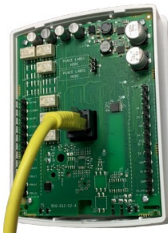
Illustration 9—Ethernet Network Connection ("E" Models)
