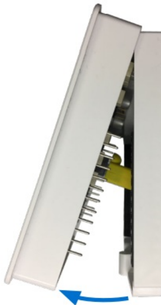
Illustration 4—Removing the Cover from the Backplate
