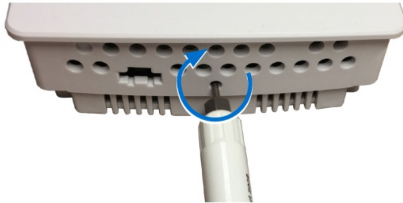
Illustration 8—Locking the Cover on the Backplate
