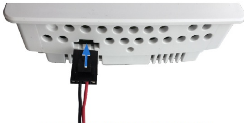
Illustration 14—MS/TP (EIA-485) Data Port
