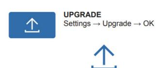
Save new firmware on a USB stick. Insert the USB stick into the USB port at the back of the projector. Follow the prompts to upgrade.
