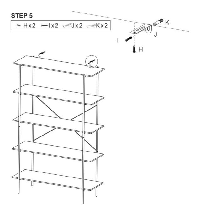
It is strongly recommended that this product is permanently fixed to the wall. Please seek professional advice if you are in doubt of what fixing device to use. Regularly check that anchors are securely maintained.
