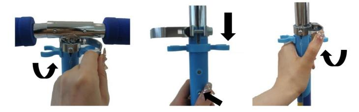
• **Step 2:** Loosen the quick release (Open position). Pull the plastic lever up and lower the steering column backward until it clips into position, then tighten the quick release (Close position).
