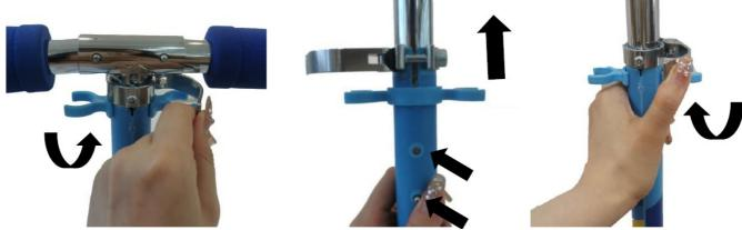
• Step 3: Press the scooter handgrip on the steering bar until the bullets are in position. Adjust the steering bar by turning off the smaller ring with a key and centre handles at right angles to the front wheel. Clamp the ring again.
