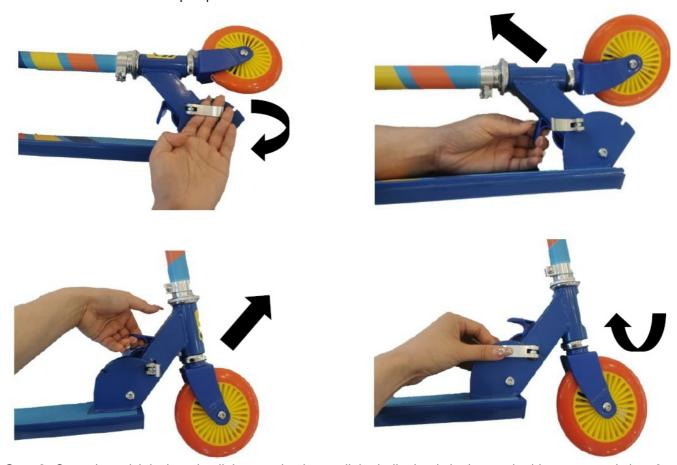
• Step 2: Open the quick lock and pull the steering bar until the bullet lands in the notch, this scooter only has 2 notches can be adjusted as below image B arrows show. Then close the quick lock. Clamp or loosen the fast lock by tightening or loosening the locknut on the open mode.
