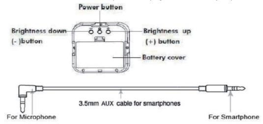
**Note:** Smartphones without a 3.5mm jack will require an adapter such as Lightning to 3.5mm for iPhones or USB-C to 3.5mm for certain Android devices (Adapters not included).
