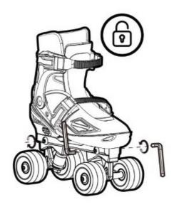
2. Separate the boot and the chassis.
