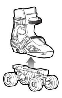
3. Switch to another chassis, insert the boot on the new chassis.
