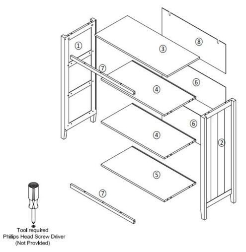
Do not tighten the screws Fully tighten screws after the final assembly steps
