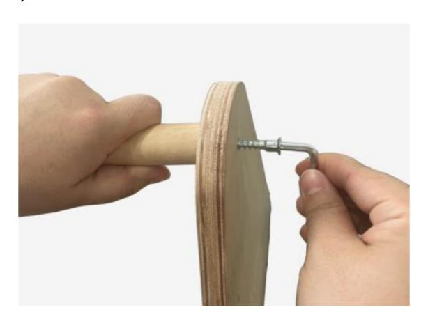
Put one end of the wooden pole to the hole on panel then take the screws and pass them through the hole, using the Allen key to tighten.
