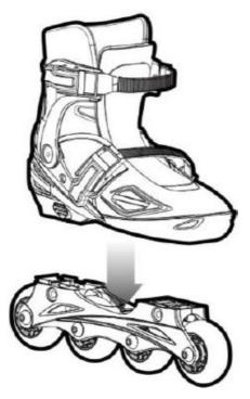
4. Tighten the screws on the new chassis.
