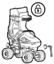
2. Separate the boot and the chassis.
