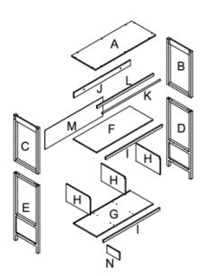
Do not tighten the screws fully during assembly. Fully tighten screws after the final assembly steps
