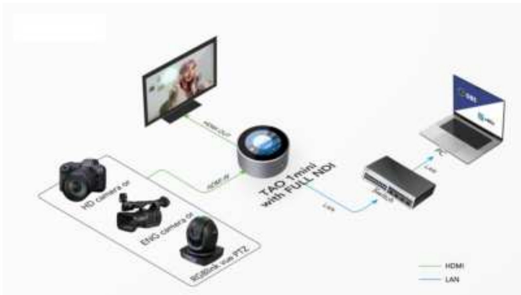
NDI Encoding Connection Diagram
