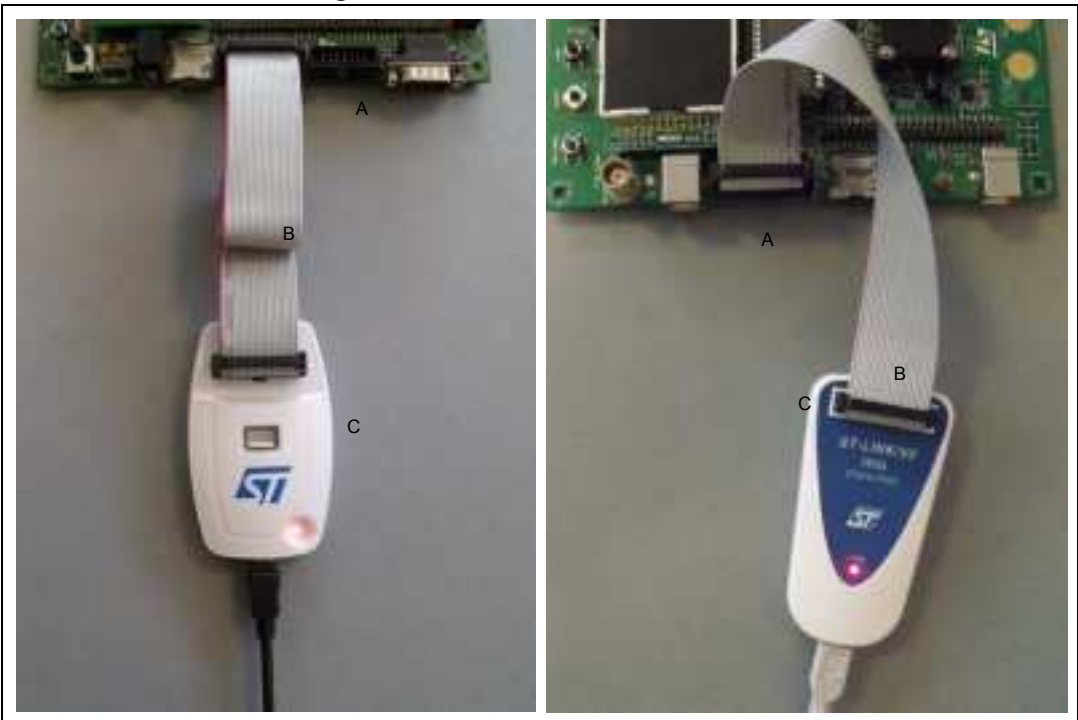
Figure 9. JTAG and SWD connection
