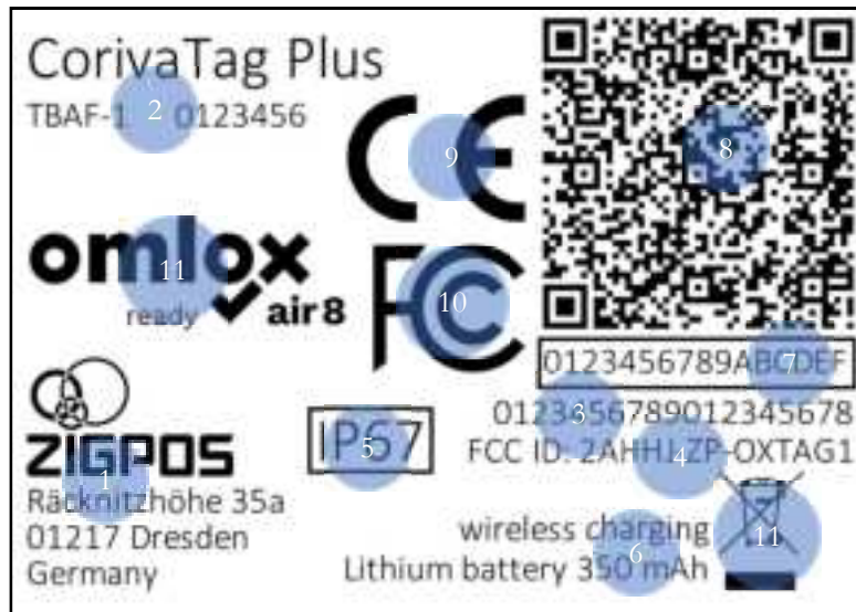
Figure 4 - Example of the CorivaTag Plus nameplate
