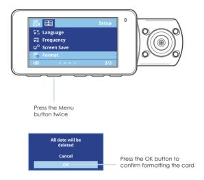
Use the  ${\bf UP}$  and  ${\bf DOWN}$  navigation buttons and go to the Format setting. Press the  ${\bf OK}$  button to confirm the selection.
