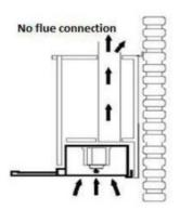
The sucked air is cleaned by passing through the grease filter and an activated carbon filter and returned to the kitchen. Carbon filters are used when it is not possible to have a chimney in the house.
