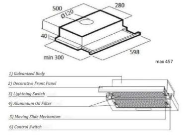
The lamp is on the left when the slide is pulled. The engine control switch is on the right when the slide is pulled.
