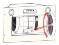
Round carbon filters are attached to the tabs on the engine cover of the product by turning them clockwise. In terms of usage and performance, it is recommended to replace the carbon filters every 3 months. Carbon filters are not washable.
