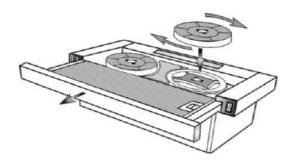
To maintain odor insulation levels, regular care of the filter is necessary. The active carbon filter should be replaced every 4 months.
