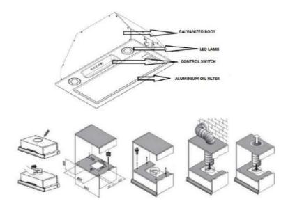
After placing the plastic flue at the motor output, attach the flexible aluminum pipe to the plastic flue. Plug the other end of the pipe into the flue hole in the wall. Example image is as follows.
