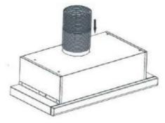
When the slide set moves, the front panel should not rub against the cabinet door. A suitable air outlet pipe should be connected to the air outlet of the aspirator in the part inside the cabinet. In cases where the flue connection pipe must be long, the use of a smooth inner surface pipe will preserve the air suction performance of the product.
