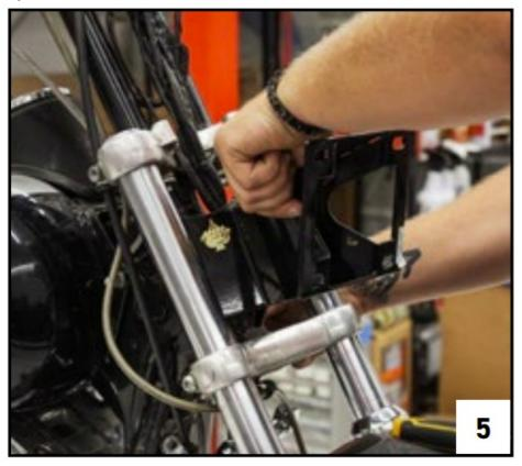
Using Hardware Bag "D" install Fairing (FIG 6) and Fairing Mount Adapter to the Neck Bracket (FIG 7). Position the Fairing Mount Adapter (FIG 8) so the notch is at the 6 o'clock down position. Snug bolts down, still allowing for
