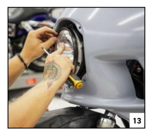
**NOTE:** Headlight adjustment screws with springs may require thread locking compound after adjustments are made.
