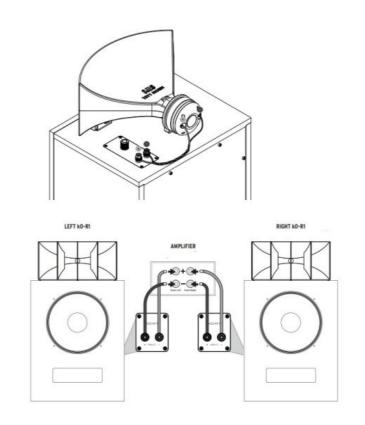
A HAND TIGHTEN ONLY, MAY INCUR DAMAGE IF TOOL IS USED
