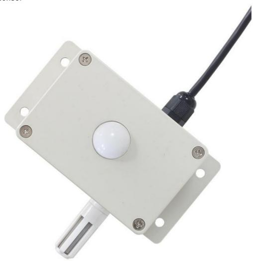
KM33B91 using the standard RS485 bus MODBUS-RTU protocol, easy access to PLC DCS, and other instruments or systems for monitoring carbon dioxide, illuminance, temperature, humidity state quantities. The internal use of high-precision sensing core and related devices to ensure high reliability and excellent long-term stability can be customized
