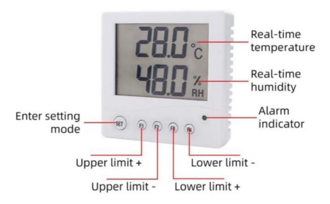
Click "SET" to enter the baud rate and change the address setting: FI and F2 change the baud rate and the def a ult is 9600, 9.6 means 9600
