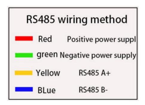
Note: power first when wiring positive and negative, after Connect the signal line
