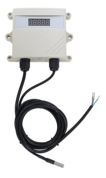
KD21B01 using the standard RS485 bus MODBUS-RTU protocol, easy access to PLC DCS and other instruments or systems for monitoring temperature state quantities. The internal use of high -precision sensing core and related devices to ensure high reliability and excellent long-term stability, can be customized RS232, RS485, CAN, 4 20mA, DC0~5V\ 10V, ZIGBEE, Lora, WIFI, GPRS and other output methods.
