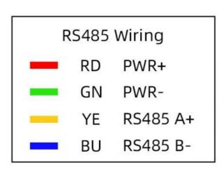
Note: When wiring, connect the positive and negative poles of the power supply first, then connect the signal wire
