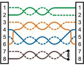
Pins 1 and 2 on the Near end are connected to Pins 2 and 1 on the Far End.
