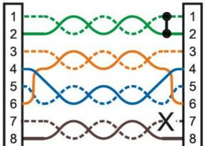
The 1-2 pair pins are shorted together and the 7-8 pair is open. The SHORT LED and OPEN LED will illuminate simultaneously.
