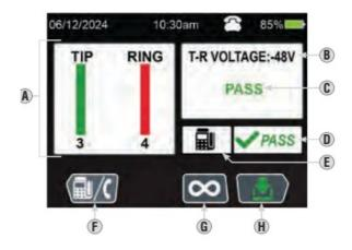
• A. Wiremap (will also display any faults detected)
