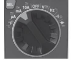
3. For  $\mu A$  DC currents <400 $\mu A$ : Insert RED test lead into V jack 5 , and BLACK test lead into COM jack 4 , and rotate function selector switch 2 to the  $\mu A$  AC/DC setting
