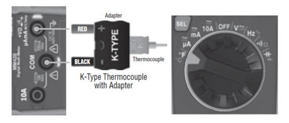
Remove thermocouple before switching meter to other measurement functions. The thermocouple included with the original purchase is suitable for temperatures below 356°F / 180°C only. To measure higher temperatures, a K-type thermocouple with the appropriate measurement range should be used.
