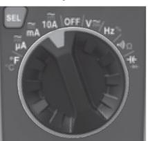
2. For mA AC/DC currents <400mA: Insert RED test lead into V jack 5, and BLACK test lead into COM jack 4, and rotate function selector switch 2 to the mA AC/DC setting.
