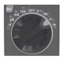
**NOTE**: When in a Resistance setting and the test leads are open (not connected across a resistor), or when a failed resistor is under test, the display will indicate O.L. This is normal DO NOT attempt to measure resistance on a live circuit.
