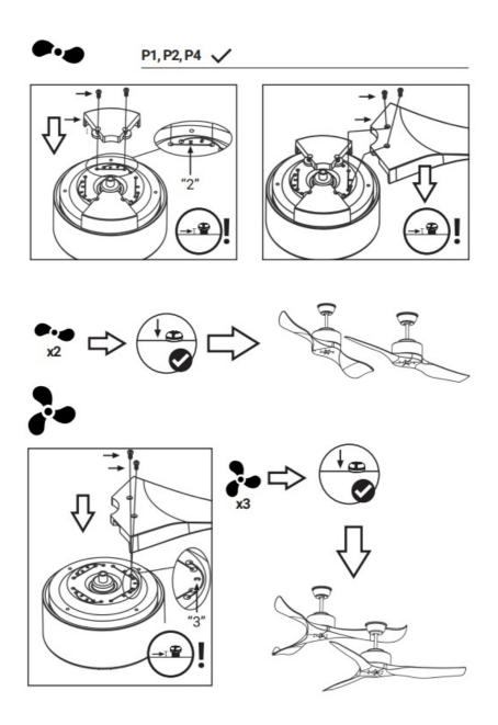
**ATTENTION!** Be careful when assembling the parts, only one unassembled item can slightly unbalance the fan. Please do not forget a single element, screws, washers.
