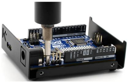
3. Close the lid and tighten the 4 countersunk screws.
