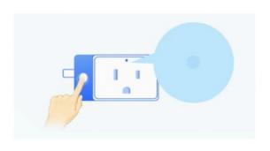
Press and hold the power button for 5 seconds until the Indicator is flashing
