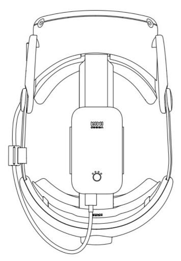
4. We recommend using the VR original adapter and cable to charge this power bank, or other qualified power adapters and cables certified with the fast charging protocol. The battery indicator flashes for the current battery level when charging the power bank.
