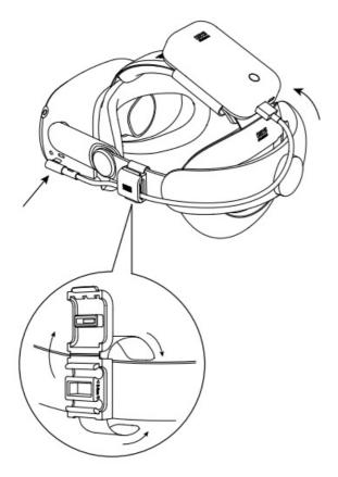
3. The power bank will charge the headset immediately once the cable is connected. During this period, the battery indicators will stay on and go off as the battery level decreases. (Please note that the switch only activates the battery indicator light and does not turn the battery on or off.)
