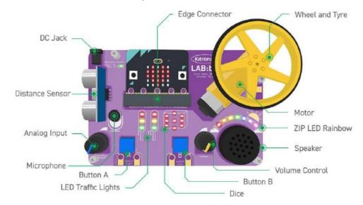
The Primary Computing Pack utilise the BBC micro:bit and our LAB:bit
