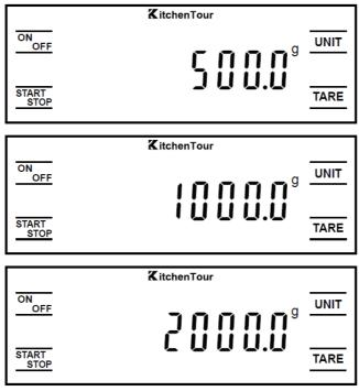
Follow the on-screen prompts to place the weights in sequence to complete the calibration process. Ready to use as soon as the calibration process is completed.
