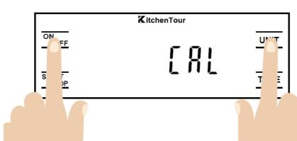
Press four buttons on/off, start, unit, tare at the same time in the off state. Release until CAL appears.
