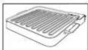
+Powered Attachment Base Pan and Heating Element
