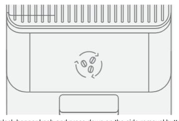
2. Remove Bean Hopper: Unlock hopper knob and press down on the side removal button.
