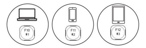
• The keyboard supports auto-reconnect. It will automatically connect to the previous device when you turn on the keyboard. (make sure you have turned on the Bluetooth). If you connect the keyboard to two or three devices, when you turn on the keyboard, it will automatically connect to the last connected device.
