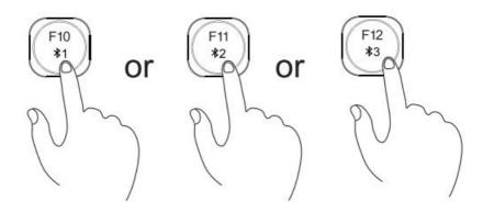
• When you successfully connected 2 or 3 devices, you can switch among the devices easily by pressing the button2/ E,
