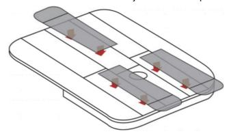
3. Install the Easyfit bracket by pressing it firmly against the wall
