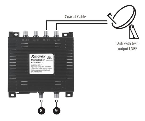
**Note:** All unused ports are to be terminated with the F-Terminators supplied.
