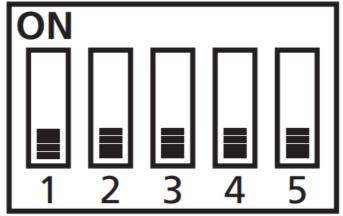
Dip Switches on the multi-stacker are switched to match up to the state/territory it is installed in.
