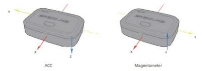
EXG Sensor Acceleration and magnetometer axis orientation. As shown in the figure below (Take TvDe-c to the left as the front):
