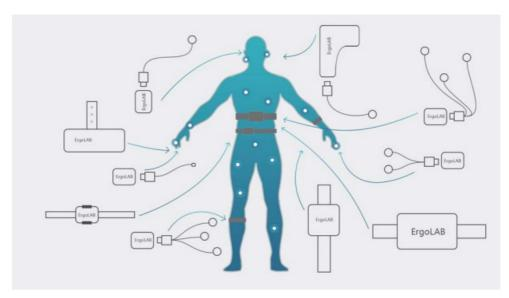
BioSensor wireless human physiological recorder adopts signal self-identification technology and is equipped with a unified collector According to research requirements, the collection line of corresponding physiological signals can be arbitrarily connected. The equipment includes PPG blood volume pulse, EDA skin electricity, RESP respiration, SKT skin temperature, FSR fingertip pressure and other indicators, each sensor can collect multiple signal indicators
