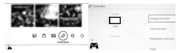
When gamepad turn off, press pair button for 2 seconds to turn on gamepad pair search mode, gamepad LED began to run with flashing lights, when single or multiple LED are always on, gameapd and console paired search success, N-S console screen appears with two gray gamepad rotating, then press the left and right gamepad L and R button together, N-S console screen gray gamepad become black gamepad Press A to complete the pairing and press HOME to exit the interface.
