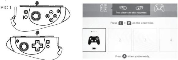
Connect the gamepad to the console again The gamepad will go to sleep if not used within 5 minutes, When the gamepad need to be reused Except TURBO button, programming button and 3D joystick, Short press other buttons to wake up reconnect and pair.
