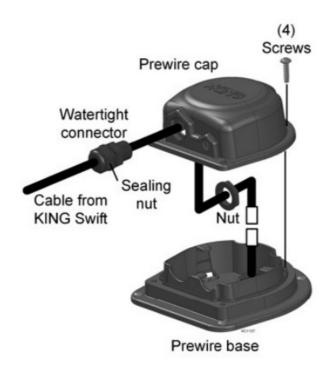
DO NOT OVER-TIGHTEN SCREWS INTO PLASTIC.
