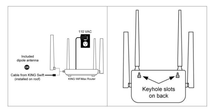
**NOTE:** You can use the keyhole slots on the back to wall mount the unit. **ANTENNAS MUST ALWAYS POINT UP.**
