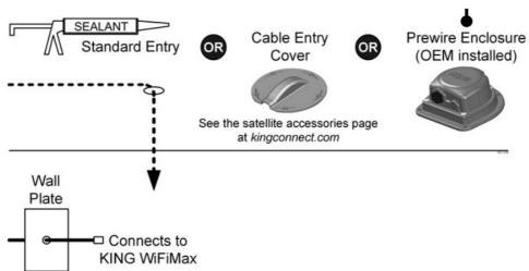
If there is a prewired enclosure on the roof, you will find a preinstalled wall plate in the vehicle. Remove this wall plate and install the included black or white wall plate.
