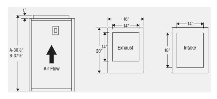
The height of the KFS furnace is the only dimension that changes. Please refer to selection chart to determine the size of the unit.
