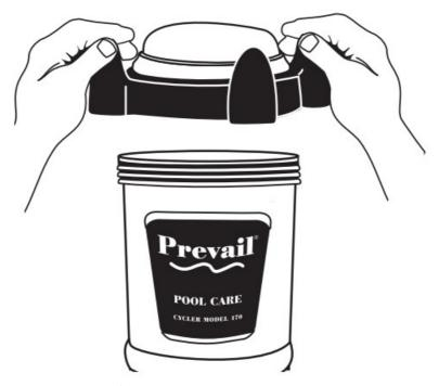
4. Unscrew knob from the front of Prevail Cycler. Allow all water to drain.
