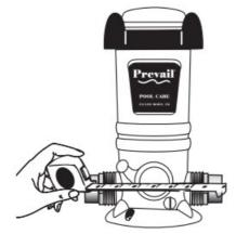
3. Following primer directions, brush primer on the inside of the adapters and to ends of pipe. Repeat this process with PVC cement following directions on that product.
