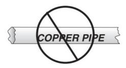
Do NOT install in copper pipe as chemical corrosion may lead to pipe failure.
