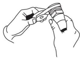
2. Screw adapters into each end of Prevail Cycler. Hand tighten. Finish tightening by turning 1 to 2 revolutions with a pipe wrench. DO NOT OVER TIGHTEN.
