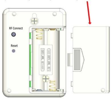
Press and hold "RF Connect" for 5 seconds enter pairing mode.
