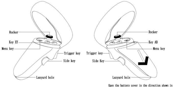
Open the battery cover in the direction shown in the figure and replace the handle battery
